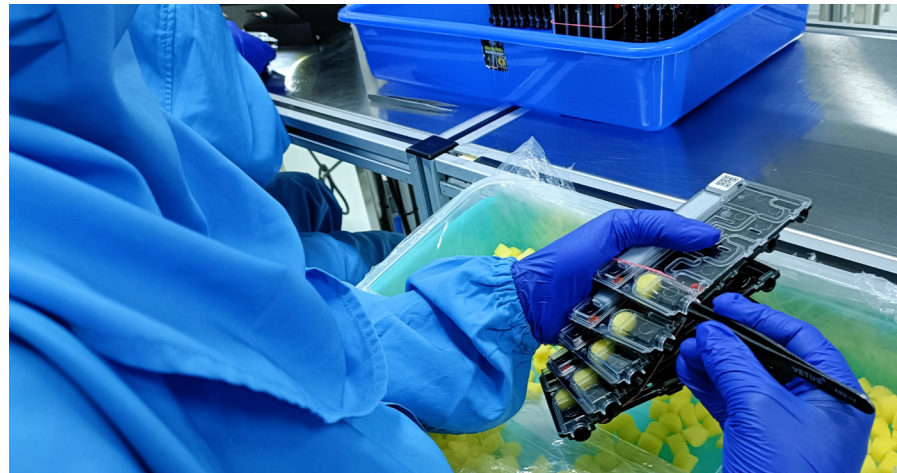
An RT-PCR test cartridge being assembled at AMTZ; (right) UHMWPE rods, used to make knee implant liners.
